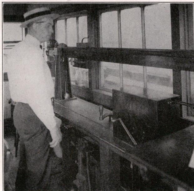
Fig. 2. Weighing a car with a Streeter-Amey recording attachment
