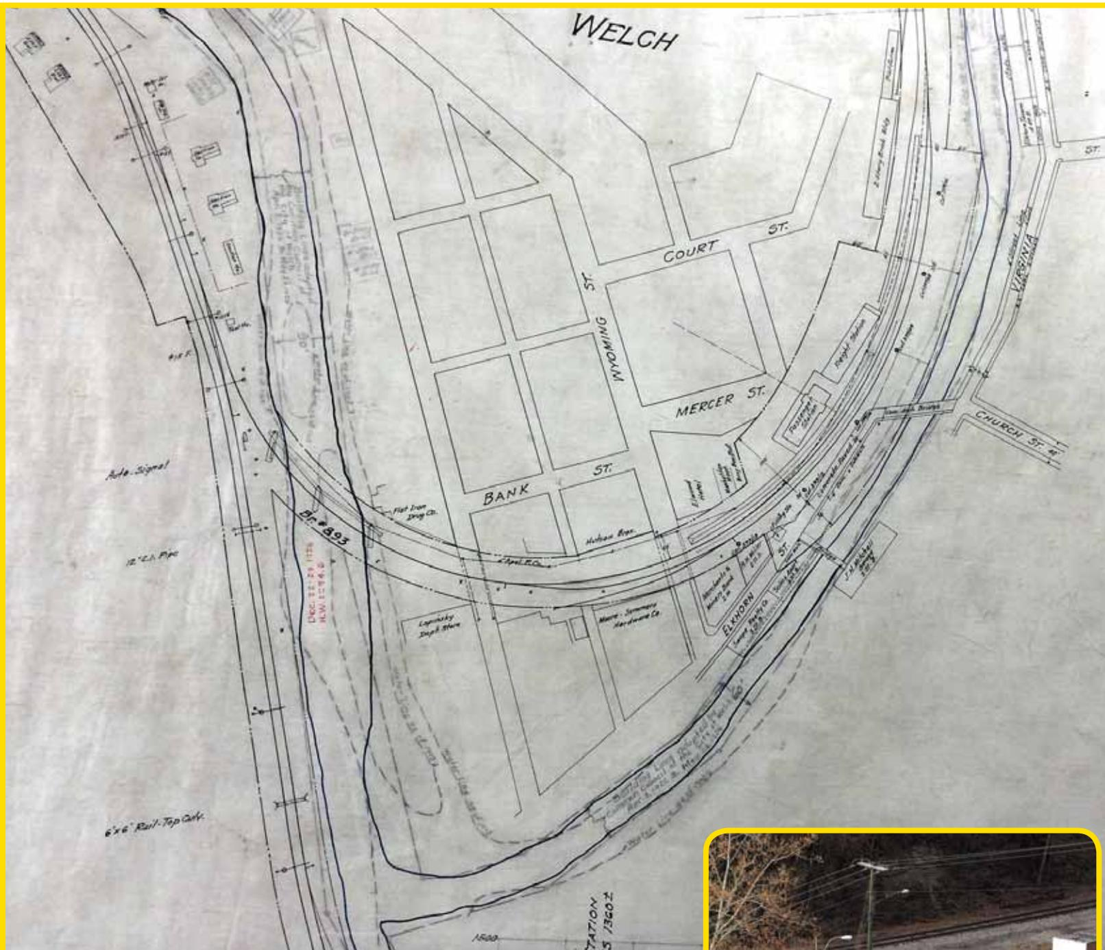
This portion of NWS Archives Drawing HS-W10017 shows the original main line through Welch as well as the track layout in Welch. Bridge No. 893 is shown center left, just downstream from the confluence of Elkhorn Creek with Tug Fork.
