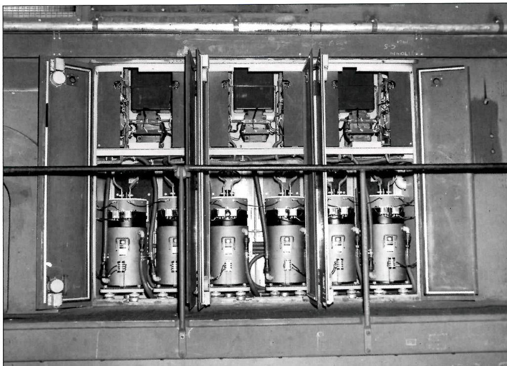
Left: One of the GE GL-6878 Ignitron tubes shown in compartment (right). GE photo. Above: Six of the 12 GE GL-6878 Ignitron tubes used on each EL-C locomotive were installed in this outside opening compartment, with doors interlocked to the power circuits, so that doors cannot be opened when the pantograph is raised. The other six tubes were similarly installed on the opposite side of the hood. GE photo.
