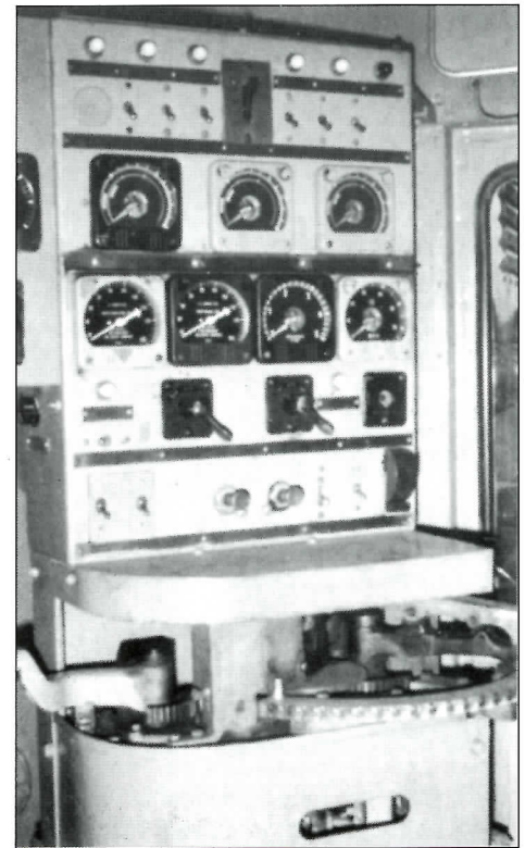
Above: This photo shows the interior cab arrangement with identifications of appliances and controls. GE Photo . Right: This EF-4 control stand was photographed after being freshly refurbished in the New Haven's shop. New Haven Railroad photo. J. W. Swanberg collection.
