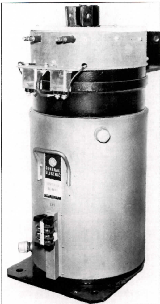
Left: One of the GE GL-6878 Ignitron tubes shown in compartment (right). GE photo. Above: Six of the 12 GE GL-6878 Ignitron tubes used on each EL-C locomotive were installed in this outside opening compartment, with doors interlocked to the power circuits, so that doors cannot be opened when the pantograph is raised. The other six tubes were similarly installed on the opposite side of the hood. GE photo.
